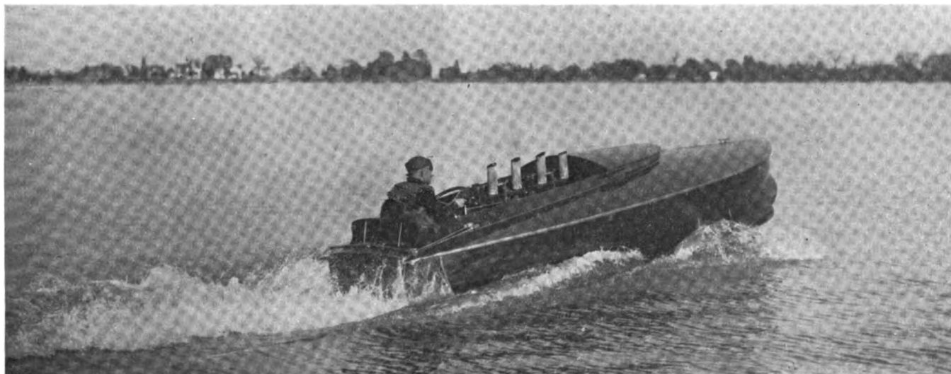
The New Tech, Designed and Built for Col. T. Coleman du Pont by Adolph E. Apel, of Atlantic City. Length 21 Ft., Beam 6½ Ft. Power Eight-Cylinder 5½ In. by 6½ In. Sterling Motor Turning at 1500 R.P.M. A Speed of Over 50 Miles per Hour, Is Said to Have Been Attained
